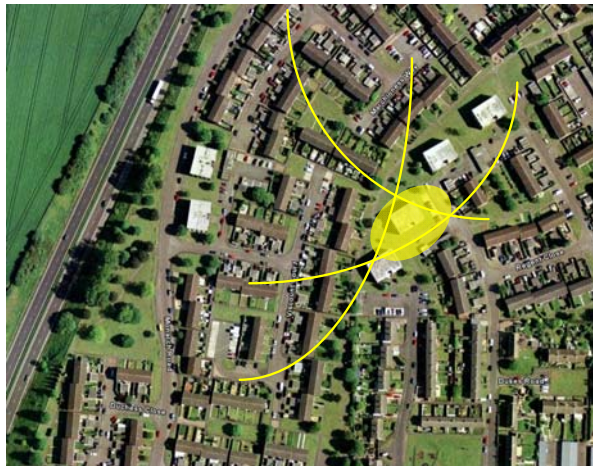
Elliptical area shows most probable interferer location at intersection of TDOA lines
